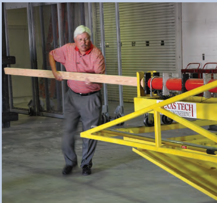
Larry Tanner, research associate at Texas Tech University's Wind Science & Engineering Research Center, prepares for testing of a storm shelter panel—the test simulates tornado conditions.
